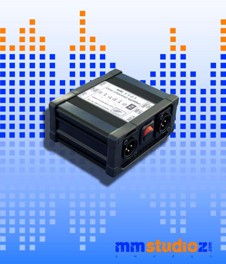
Splitter MM 1121 is a high quality professional audio signal splitter for use on stage, in studio, in OB vehicles etc. This passive splitter offers mic and line signal level splitting without coloring the signal. Input are on Combo receptacle. The direct output and two transformer isolated outputs are all on male XLR connectors.
